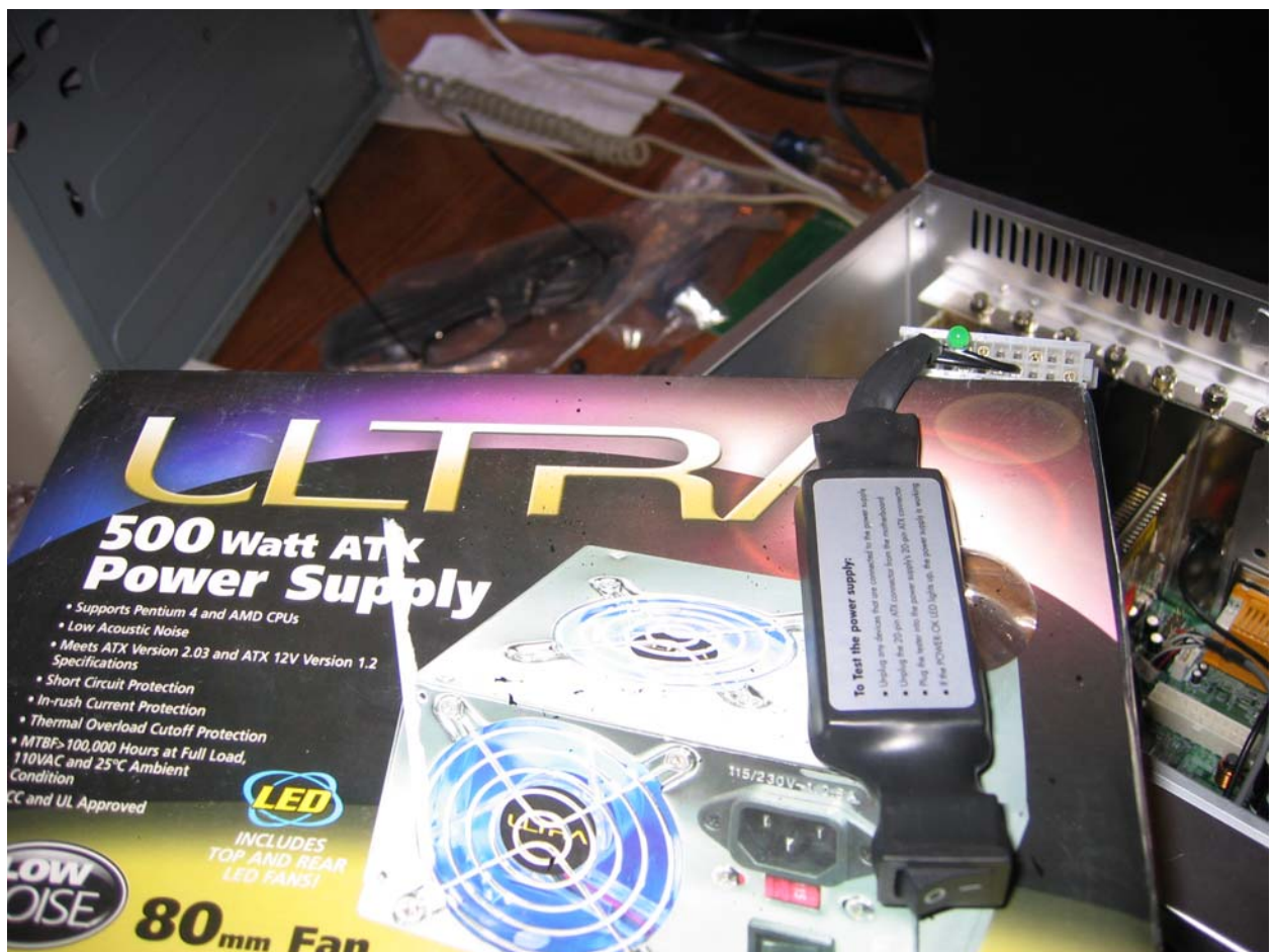
Figure 5 LED Off Indicates a Dead Power Supply. Fortunately a Spare Is On Hand.
